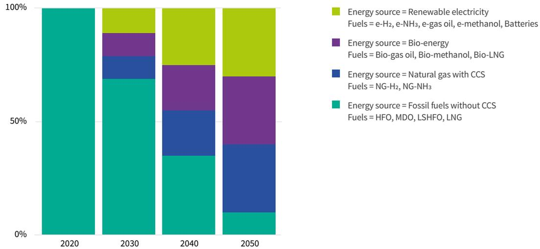
Figure 13 - Energy source and marine fuels mix assumed in **equal mix** pathway
