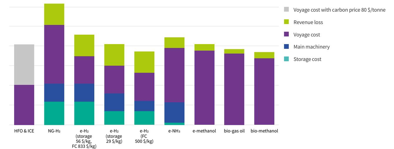
Figure 9 - Relative competitiveness of ZEVs using electro-fuels for a small-medium sized container ship
