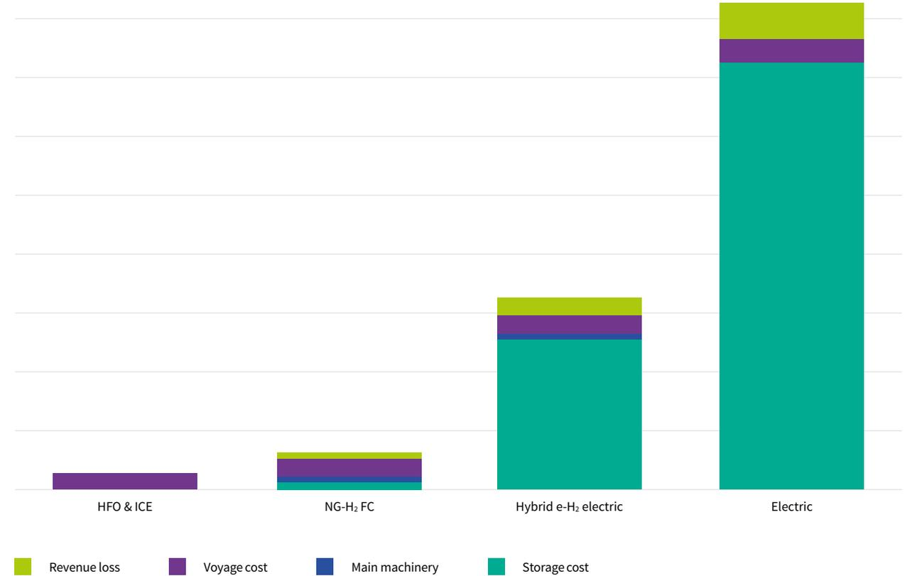
Figure 4 - Additional costs relative to the reference ships for hydrogen-hybrid and full electric with batteries ZEVs<sup>4</sup>
