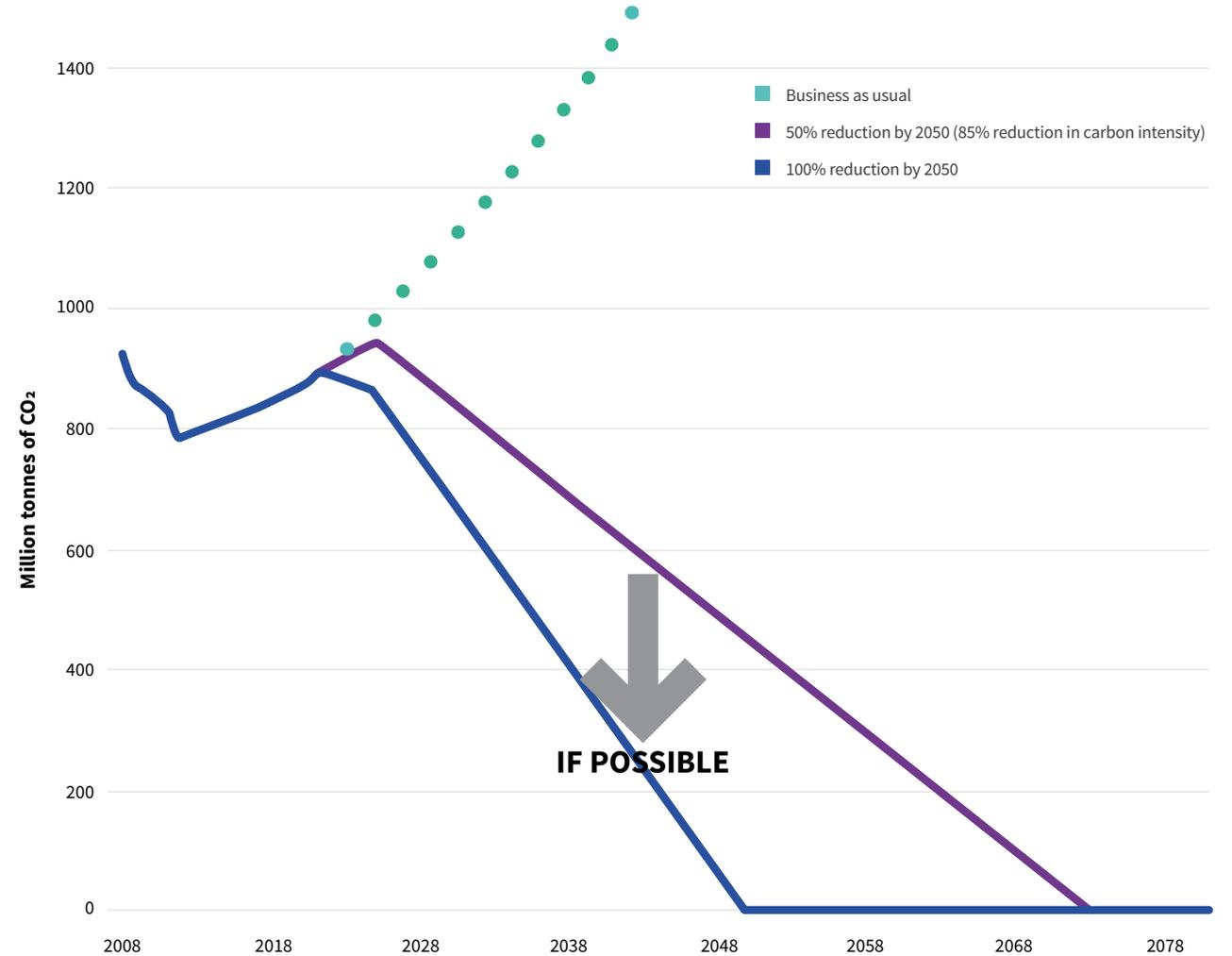
Figure 1: Carbon dioxide (CO<sub>2</sub>) reduction trajectory for international shipping in line with the IMO Initial GHG strategy
